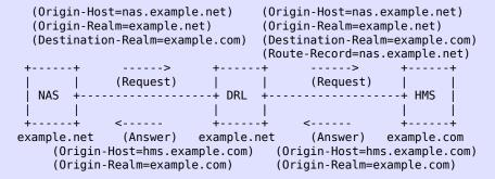
Figure 6: Routing of Diameter messages
