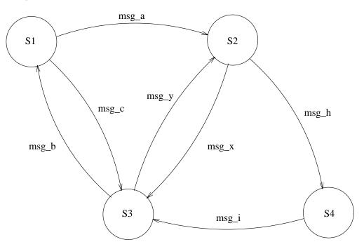
Figure 5.3 Finite state machine
