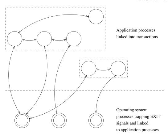
Figure 8.2 Operating system and application processes
