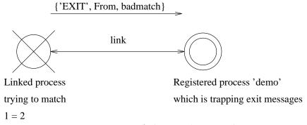
Figure 7.5 Process failing with a match error
