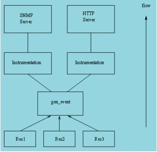
Figure 1.4: Notification Handling
