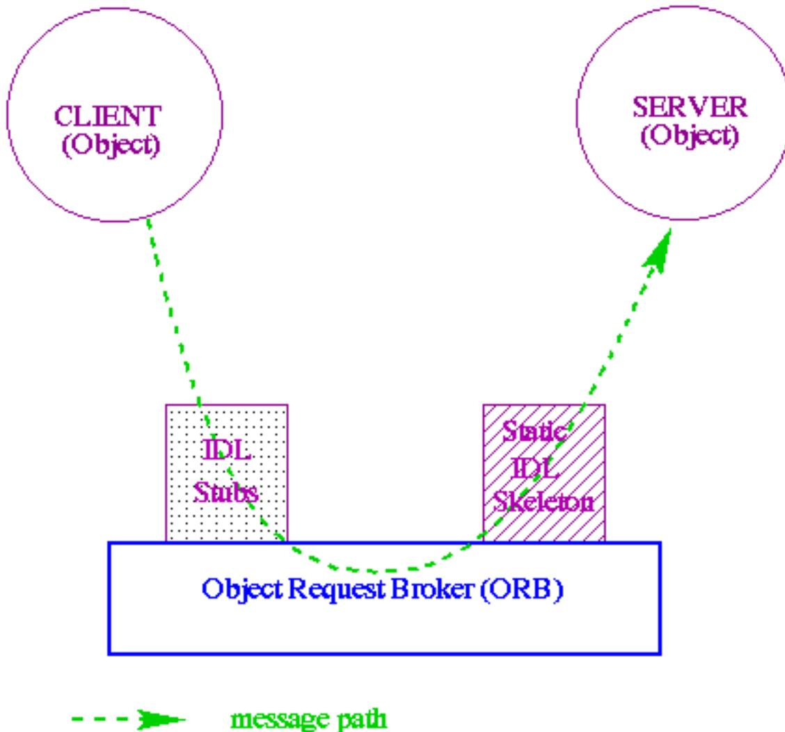
Figure 3.1: Figure 1: How the Object Request Broker works.
