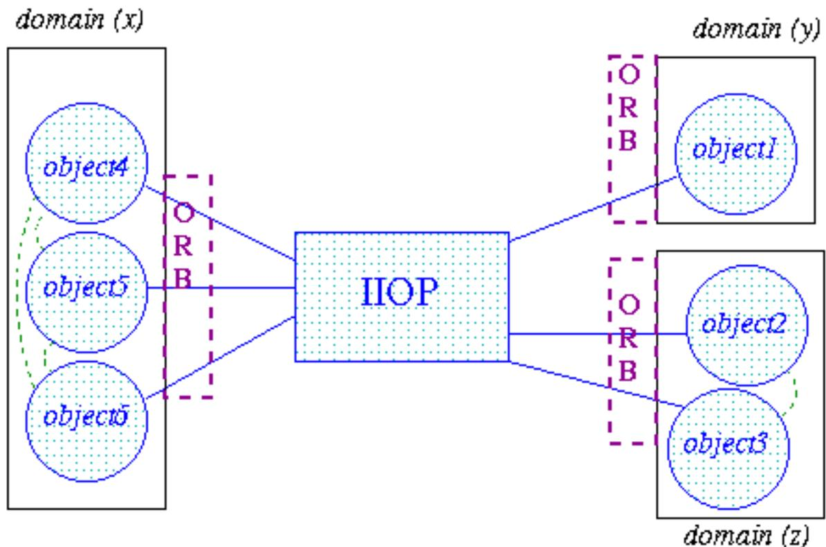
Figure 3.2: Figure 2: IIOP communication between domains and objects.
