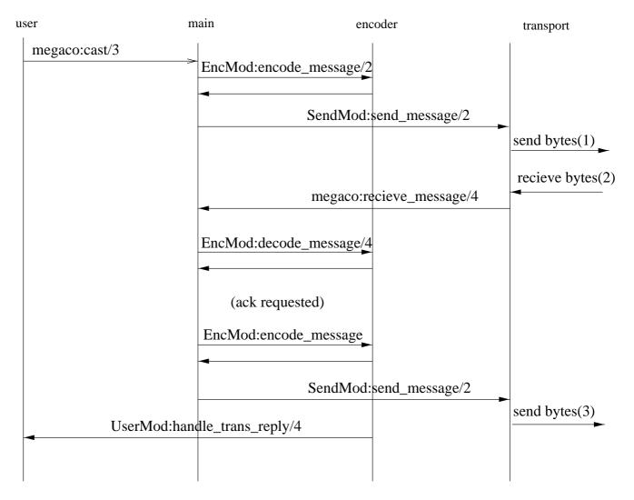
Figure 1.4: Message Call Flow (originating side)
