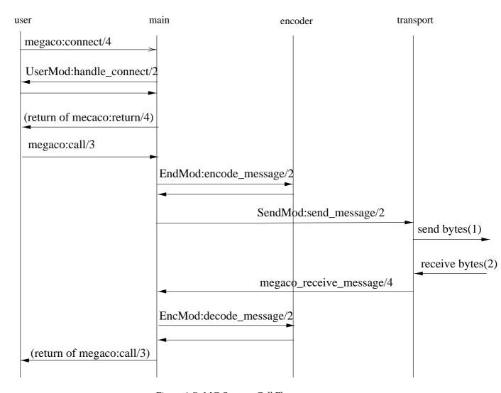
Figure 1.7: MG Startup Call Flow
